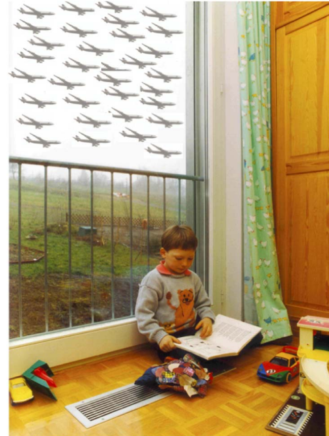
1 plane, window tilted = 45 dBA (= 32 planes, window closed)
